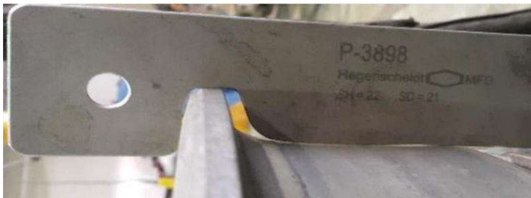
Figure 7: CNR profile defective flange thinning
