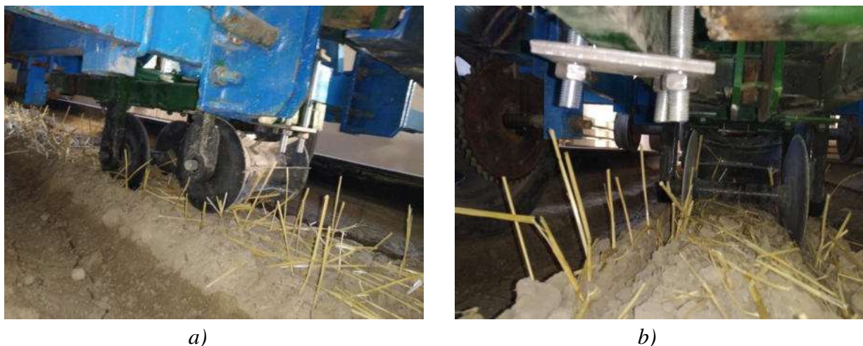
Figure 4. Installation of the disc blade in the soil channel (a) and the process of cutting the disc blade from the ridge marked strip (b).
