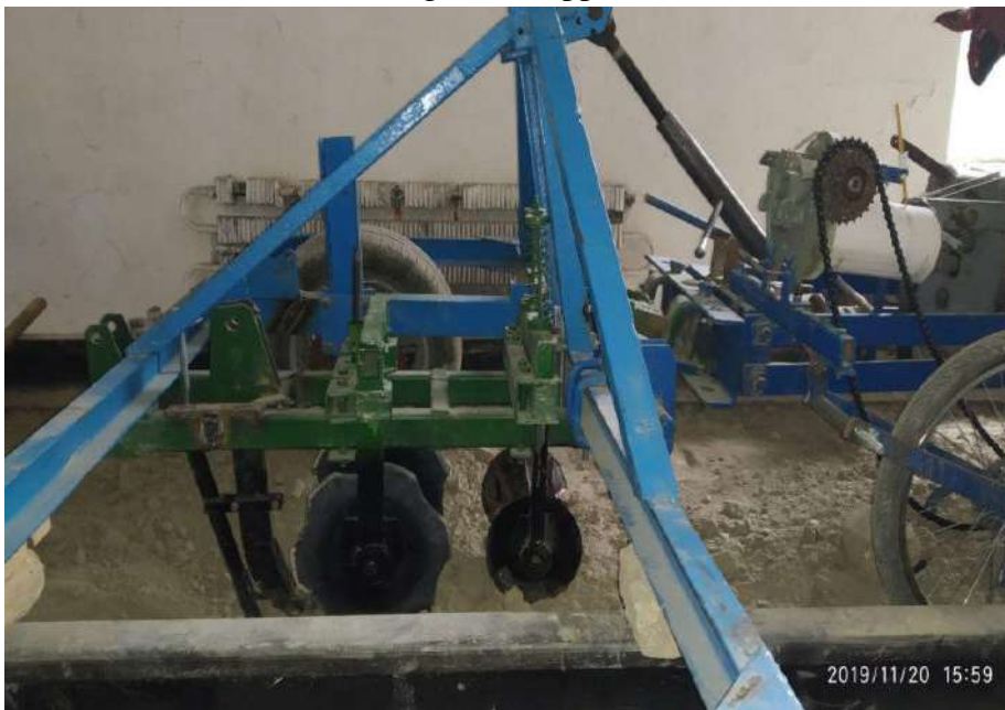
Figure 5. Installation of the ripper on the section
