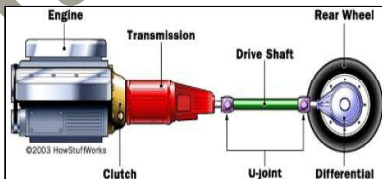
**Figure. 1 Conventional one piece drive shaft arrangements for rear wheel vehicle driving system**
