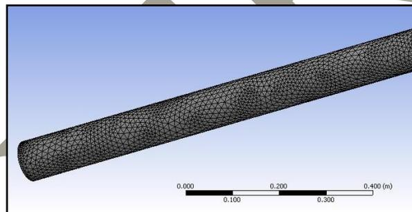
**Figure 2. Finite element model of E glass/Epoxy shaft**
