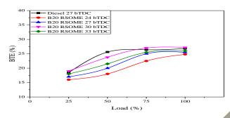
Figure 4. Variation of BTE with Load for RSOME at Different Injection Timing
