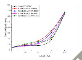
Figure 8. Variation of Smoke Opacity Emissions with Load for RSOME at Different Injection Timings
