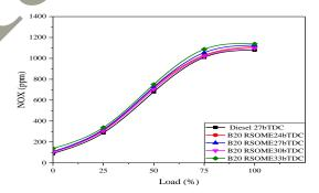
Figure 7. Variation of NO<sub>x</sub> Emissions with Load for RSOME at Different Injection Timing
