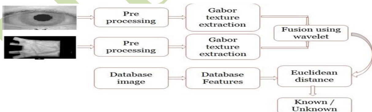
Fig. 1 Typical Block Diagram of a Multimodal Biometrics
