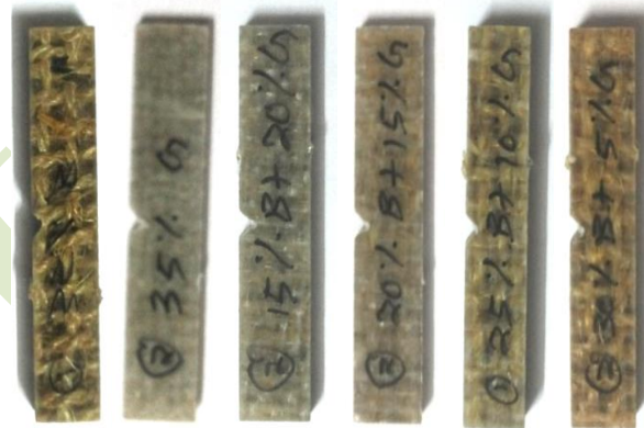
Fig. 4 SENB test specimen before fracture
