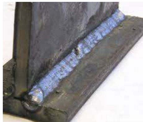
Fig.5: Design of transverse fillet welded joint
