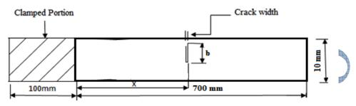
Fig.4 Cracked Square Beam Specimen
