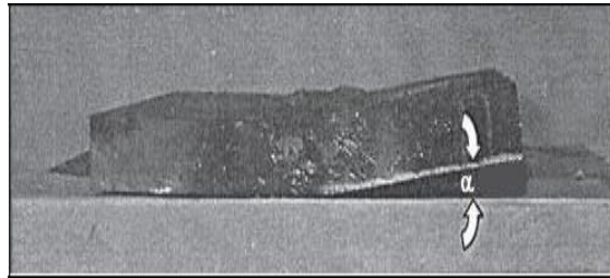
Fig 4 Angular Distortion of the Specimen during Experiment
