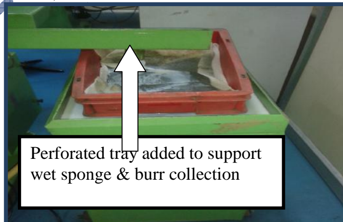
Fig1.4: Old filtration system with sponge & perforated tray.
