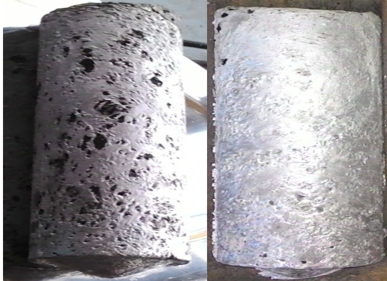
Fig.6 Agglomeration of CNT on Surface of Cast Specimen.
