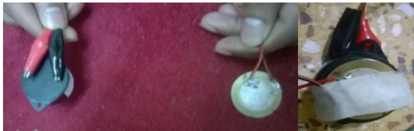
Figure2: Piezobuzzer and piezodisc are (a) kept in air (b) placed on each other
