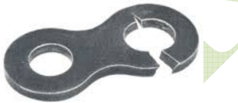
Fig.1. Failure of chain link
