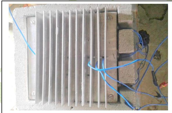
Plate fin array[H = 3cm, L= 150mm,S =6mm]
