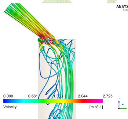
**Velocity streamline for 10mm valve lift**
