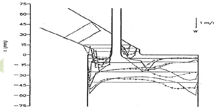
**Fig.6.1 Comparison of predicted and experimental results for valve lift 10mm performed in previous study**
