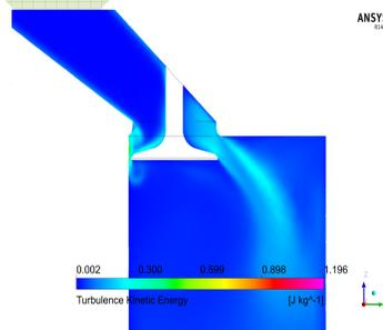
**Turbulent kinetic energy profile for 10mm valve lift**
