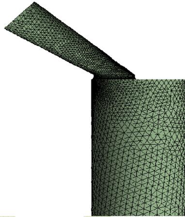
Fig 3.1 Meshed model in FLUENT
