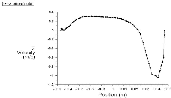
**Fig.6.2.3 Prediction of velocity in  $z=-45\text{mm}$  for valve lift 10mm in present study**
