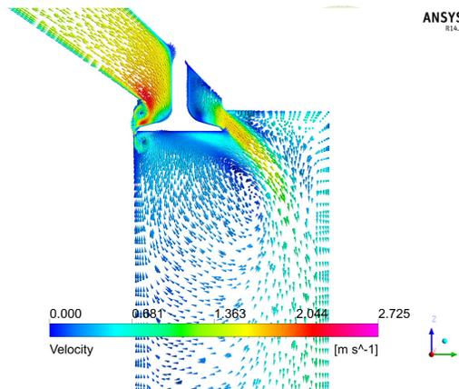
**Velocity contour profile for 10mm valve lift**
