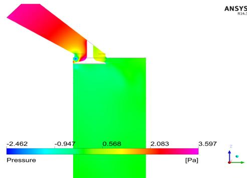
**Pressure profile for 10mm valve lift**
