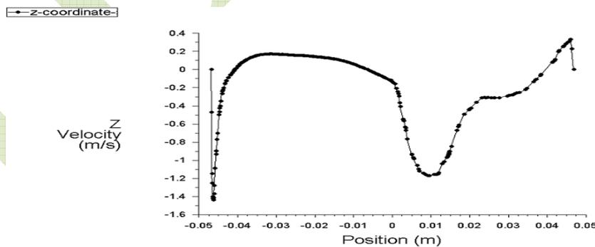
**Fig 6.2.1 Prediction of velocity in z=-15mm for valve lift 10mm in present study**
