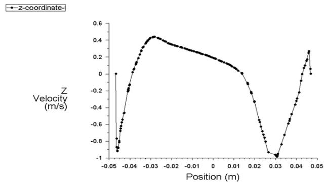
**Fig.6.2.2 Prediction of velocity in  $z=-30\text{mm}$  for valve lift 10mm in present study**
