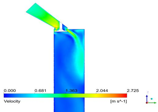
**Velocity profile for 10mm valve lift**
