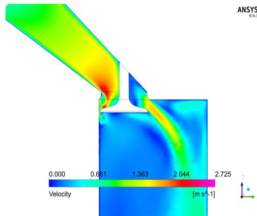
**Velocity profile for 10mm valve lift**
