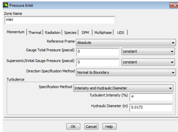
**Figure.5. 1 Pressure inlet boundary conditions windows**
