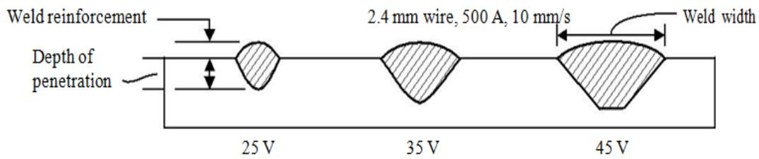
**Figure 6. Weld Bead**
