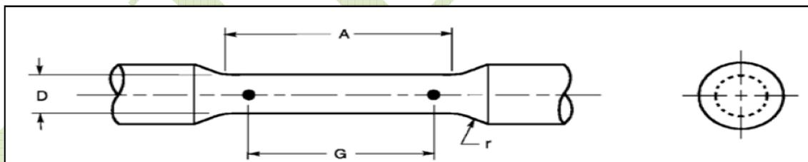
Figure 8 Weld specimen
