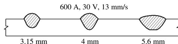
**Figure 7. Effect of electrode size on bead geometry**
