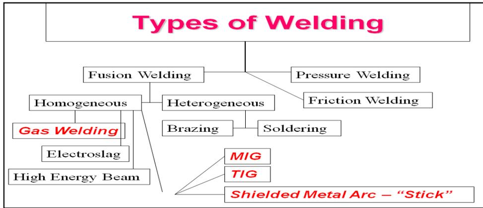
**Figure 1. Types of Welding**
