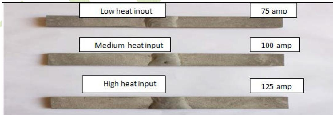
**Figure 9** Weld Specimen after welding
