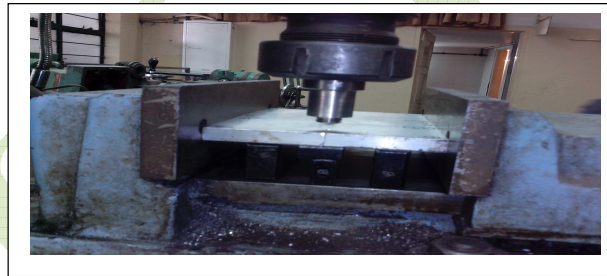
Figure 4: Experimental Setup for Friction Stir Welding
