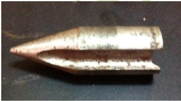
Fig. 2 (A) Nozzle or Rocket (Used in Pneumatic Injection Moulding Machine) (b) Nozzle with barrel in processing position Source: Ref.[ 1]
