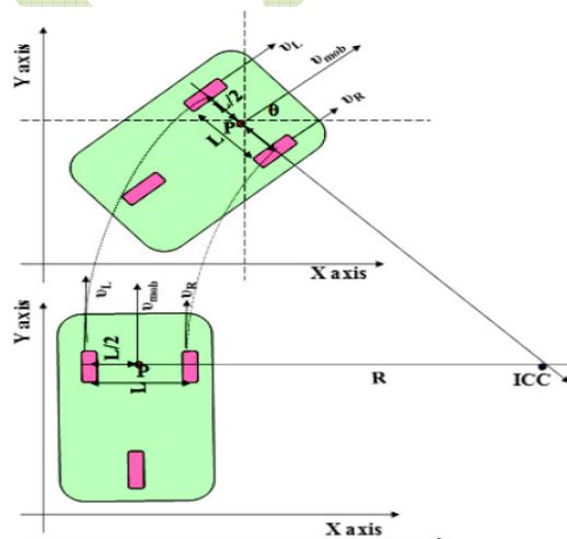
**Figure 5: Differential Drive Motion.**
