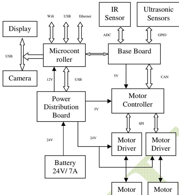
**Figure 2: Block diagram of Hardware**
