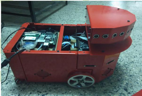
**Figure 6: Manufactured Differential Drive Robot.**
