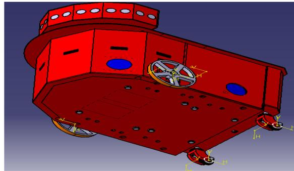
**Figure 3: Wheel configuration of the Robot.**
