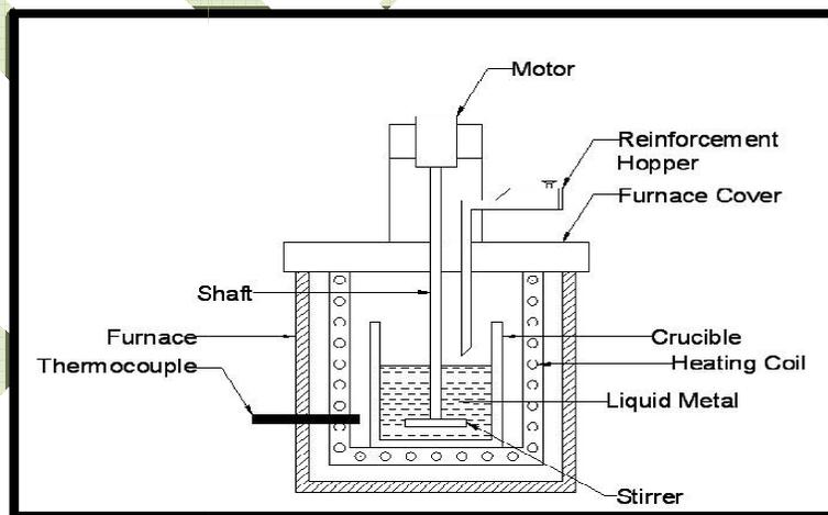
Fig 1 Schematic view of stir casting setup
