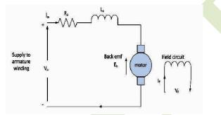
Figure 1: Schematic Diagram of a separately excited DC Motor
