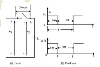
Figure 3: Operation of chopper and its waveforms
