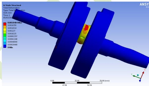
**Fig 6 Total Deformation**
