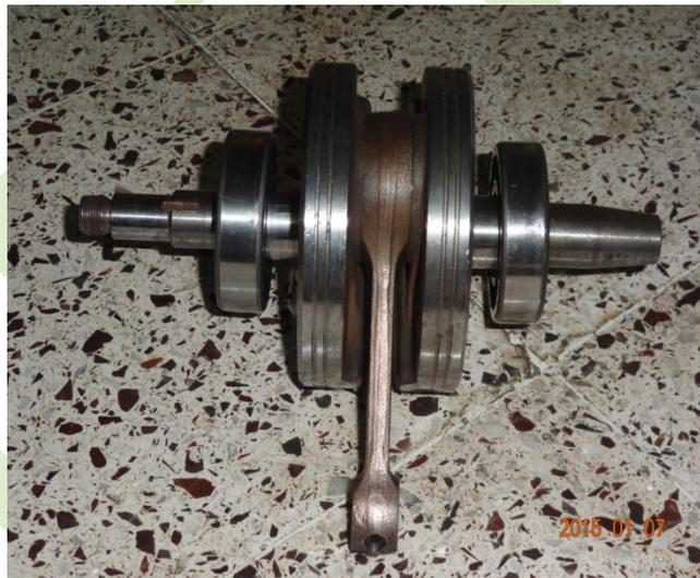
**Fig 1: Single Cylinder Petrol Engine Crankshaft**
