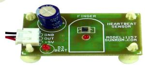
Fig 3. Heart rate sensor module
