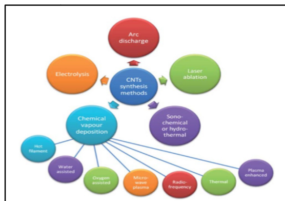
Fig. 1 Methods of CNT synthesis. [4]
