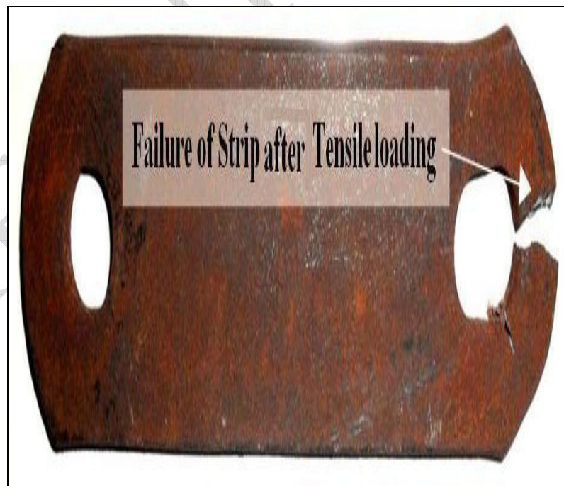
Fig.4. Failure of strip
