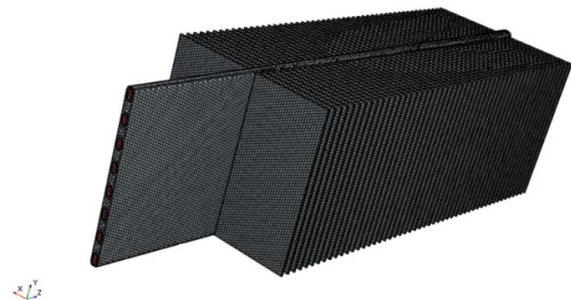
Fig. 5 Mesh Generation of Heat Exchanger
