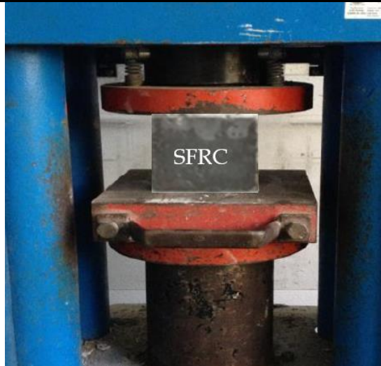
Figure 3. Compressive strength test on Concrete cube samples
