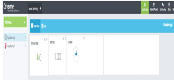
Fig-5:- Water-pump indication output in cayenne
