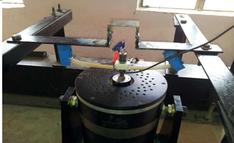
Fig.1b Experimental Setup for Dynamic Analysis of glass fiber Leaf Spring
