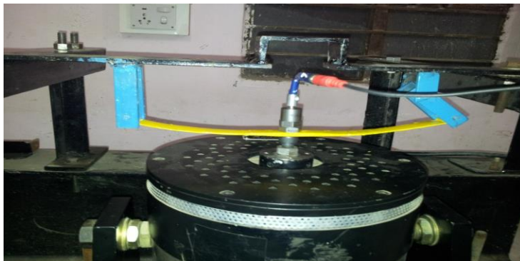
Fig.1a Experimental Setup for Dynamic Analysis of Steel Leaf Spring
