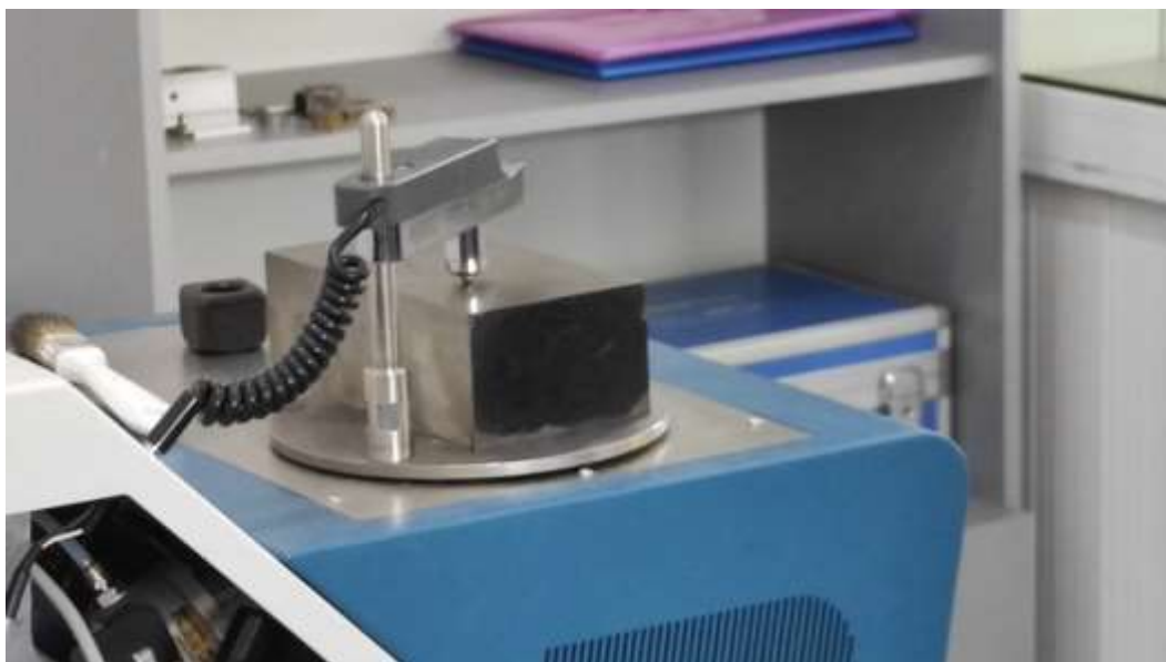
2-picture. Chemical analysis process of bulk detail in uzstandard laboratory (spectrometer)
