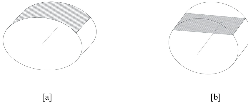
Fig.2: Representation of Radial Cross-sectional Area in Curved and Simplified View The geometry of the flow control metering notch of the spool is shown in figure below.
