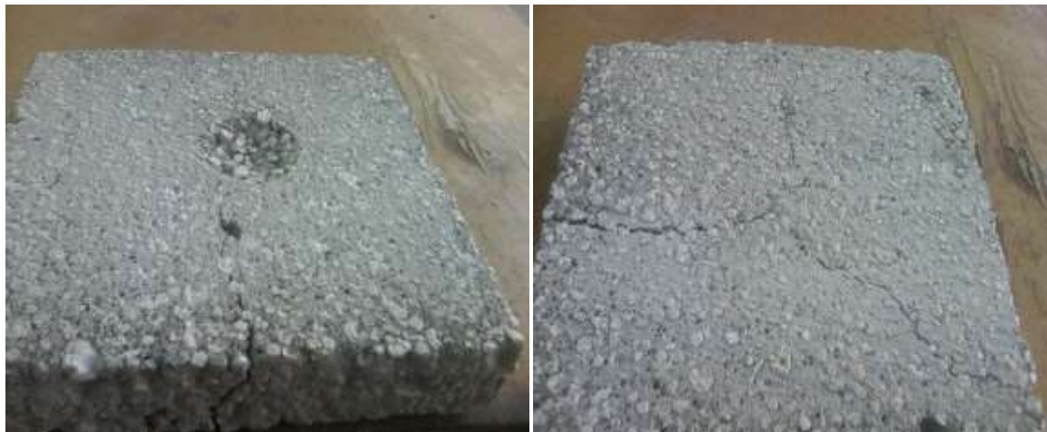
Fig 2. The nature of the destruction of the control (H-4) sample
