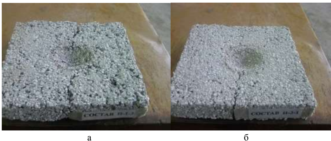
Fig 3. The nature of the destruction of samples H-1 (a) and H-3 (b)
