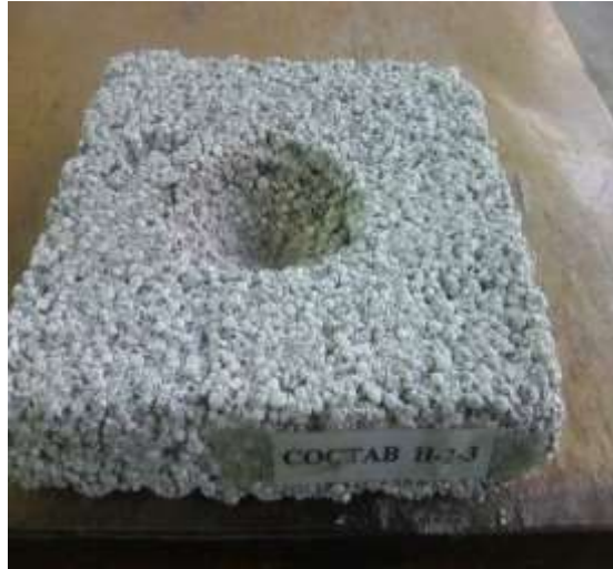
Fig 4. The appearance of the sample H-2 after the impact strength test
