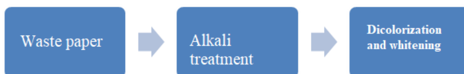
Figure 4. The sequence of cleaning waste paper from printing ink.
