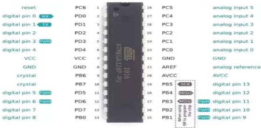
Figure 4 (a) : A 28-pin ATMEGA 328P-PU micro-controller
