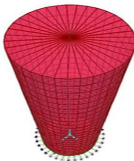
Figure 2: Steel Silo Finite Element Model without GFRP
