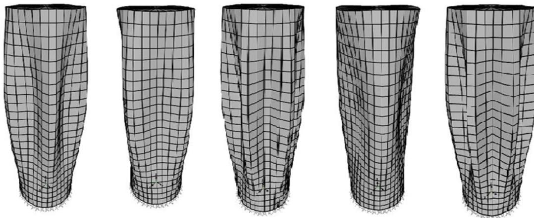
Figure 5: Respectively Mode Shapes of Steel Silo with GFRP
