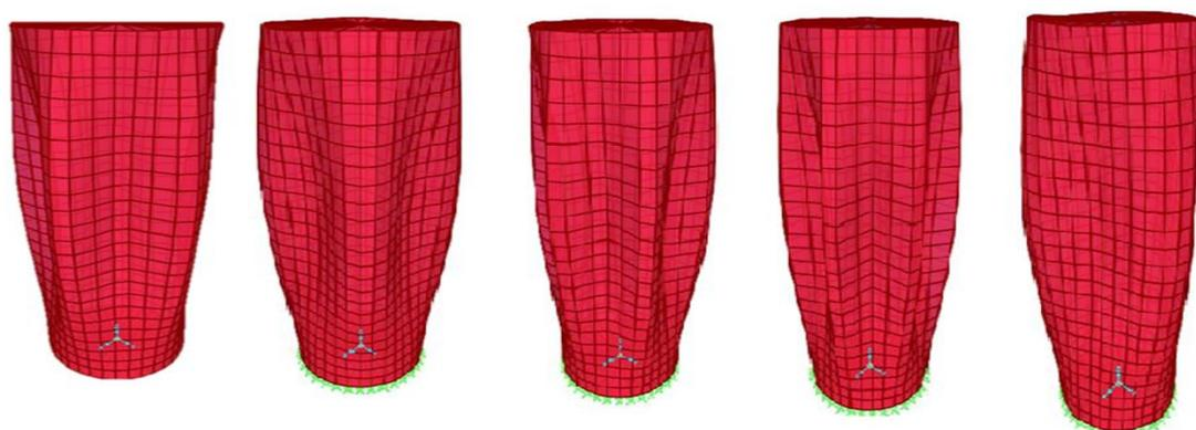
Figure 3: Respectively Mode Shapes of Steel Silo without GFRP
