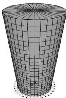
Figure 4: Steel Silo Finite Element Model with GFRP
