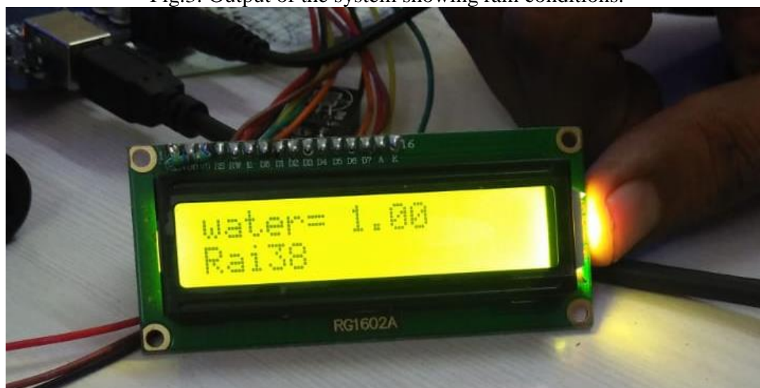
Fig.3: Output of the proposed system showing the water level of soil
