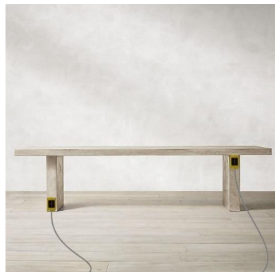
Figure 10: The accelerometer placement arrangement in Setup 2
