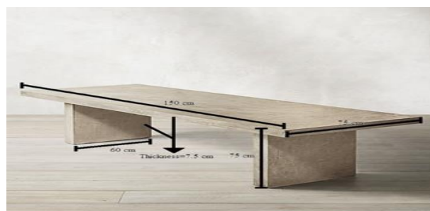
Figure 1: Dimensions of scaled concrete bridge
