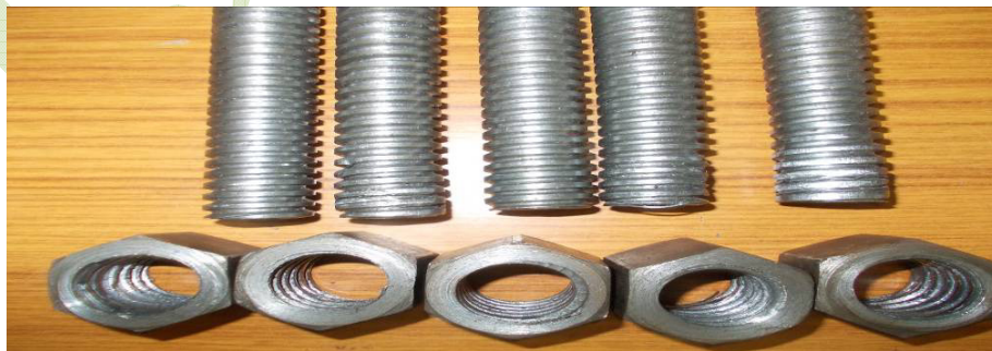
Fig: 5. five specimens of Modified Square threaded mild steel IS2062 tie rods
