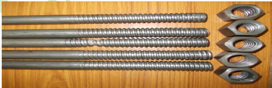
Fig: 4. five specimens of ACME threaded mild steel IS2062 tie rods
