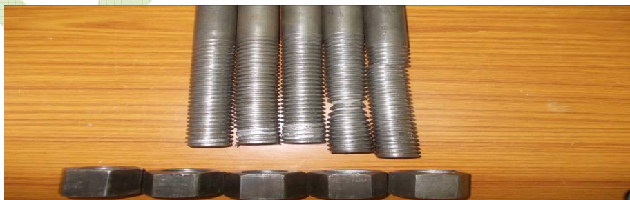
Fig: 3 five specimens of Buttress threaded mild steel IS2062 tie rods
