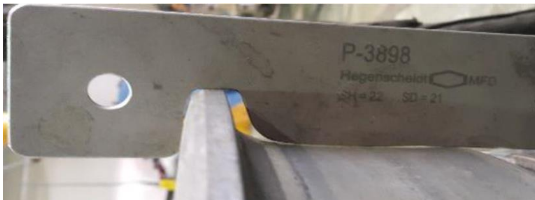
Figure 7: CNR profile defective flange thinning
