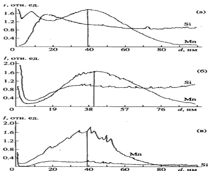
Fig. 1. Manganese distribution profiles in silicon at implantation doses  $N_0 = 5 \cdot 10^{15}$  (a),  $5 \cdot 10^{16}$  (b),  $5 \cdot 10^{17}$  ion /  $\text{cm}^2$  (c) ( $d$  is the layer depth). For samples doped with Mn at a dose of  $10\text{-}15$  ion /  $\text{cm}^2$ , the
