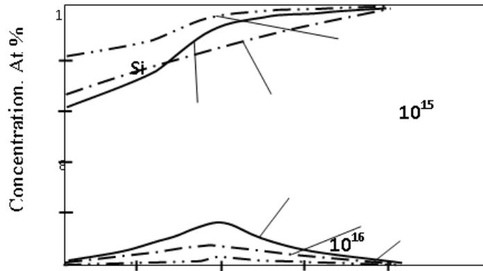
Fig. 2. Depth distribution of Mn concentration in Si at an irradiation dose of 1015 - 1017 ion / cm<sup>2</sup>
