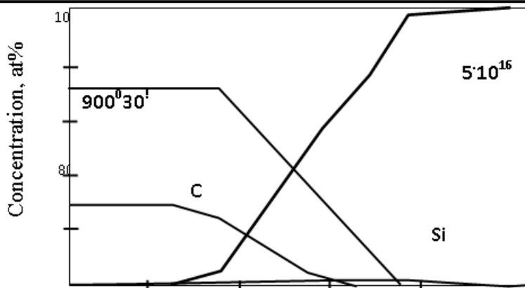
Fig. 4. Depth distribution of Mn concentration in Si at an irradiation dose of  $10^{16}$  ions /  $\text{cm}^2$  after annealing at a temperature of  $9000^\circ\text{C}$  for 30 minutes
