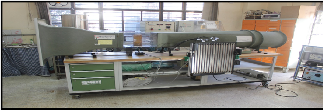
Plate (3b) The Laboratory Wind Tunnel with the Second Model. Plate (3) Photographs Showing the Laboratory Wind Tunnel with: (A) First Model, (B) Second Model.
