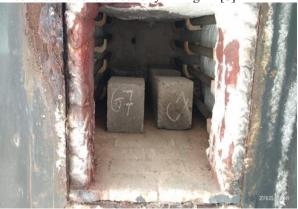
Fig. 2 Concrete Specimens kept in furnace for checking temperature effect
