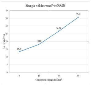
Fig. 1 Graphical Representation of strength variation with increase in % of GGBS
