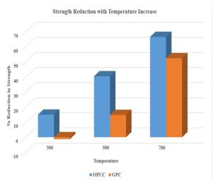
Fig.4 Graphical Representation of Strength Reduction with Temperature
