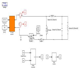
Fig.5 (a). Simulink model for buck mode.
