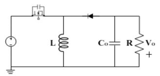
Fig.1.Circuit diagram of the single switch buck-boost converter with DC source.
