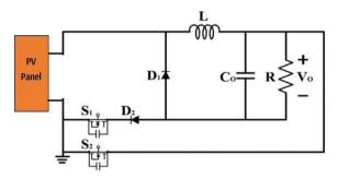
Fig.3. Circuit diagram of two switch buck-boost converter with PV system.
