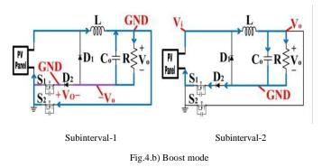
**Subinterval 1-** In case of boost mode operation switch  $S_1$  made on continuously and switch  $S_2$  is use for switching as there are two paths for current one is through load and another is through switch  $S_2$ . Here we can control the voltage across the load by controlling switching of  $S_2$ . In this interval total input voltage from PV system is appear across the load.
