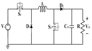
Fig.2. Circuit diagram of two switch buck-boost converter with DC source.
