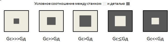
Fig. 5. Geometric model for predicting the evolution of machines of various sizes ( G_c -weight of the machine, G_d -weight of the part)
