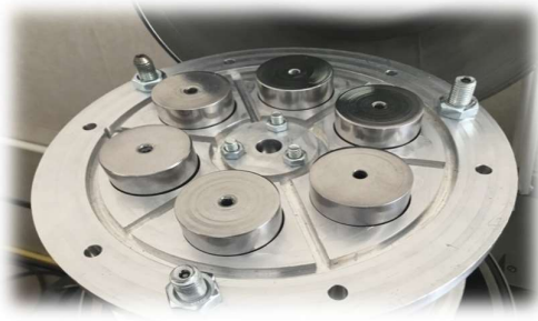
Figure 1 - Vacuum post VUP-5 with a special insert for testing materials for gas evolution
