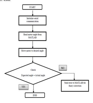
Fig. 5 Flowchart of Microcontroller code
