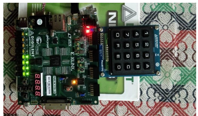
Fig. 5 FPGA and keypad interfacing
