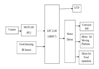
Fig. 1. Block diagram Of Automatic Fruit Sorting and Quality Analyzer
