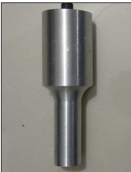
Fig. 3. Titanium (Grade 5) Welding Horn
