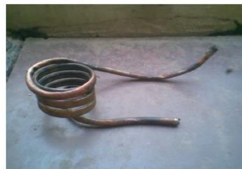
Fig.10 Copper tube after bending
