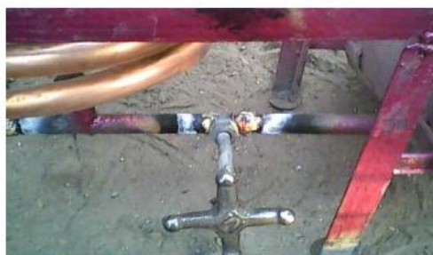
Fig.8 After brazing process
