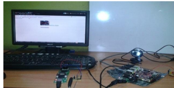
Fig. 12 Web page sent by Target board to the remote Client
